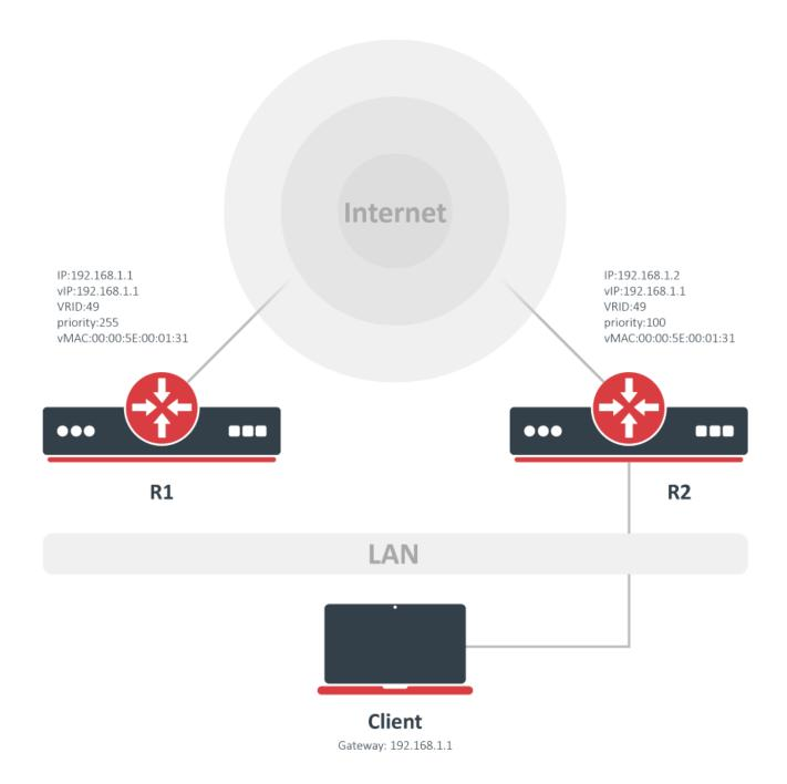
The purpose of the VRRP is to communicate to all VRRP routers associated with the Virtual Router ID and support router redundancy through a prioritized election process among them.
