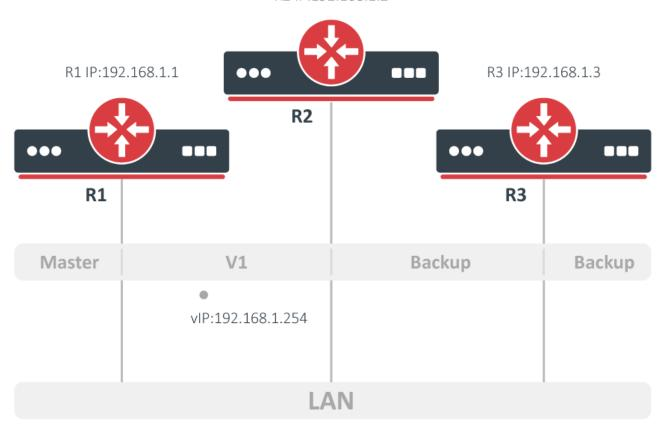
Virtual IP associated with VR must be identical and set on all VR nodes. All virtual and real addresses should be from the same network.
