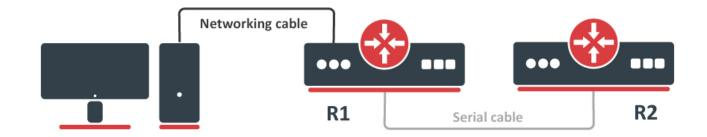
Routers R1 and R2 are connected with serial cable and PC is connected to R1 via ethernet. Lets say we want to access router R2 via serial cable from our PC. To do this you have to set up serial interface proxy on R1. It can be done by feature called **special-login**.
