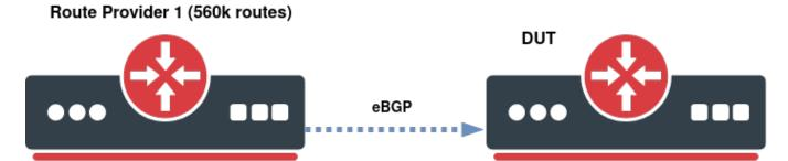
DUT establishes a connection to simulated upstream peers, receives routes, and installs them in FIB.
