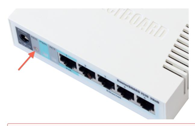
If you have set up a Protected bootloader, then the reset button's behavior is changed. Make sure you remember the settings you used to set up the Protected bootloader, otherwise you will not be able to use Eterboot mode and will not be able to reset your device.
