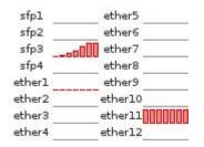
All interface graph screen shows the RX/TX bandwidth usage about all interfaces. The max values are calculated like this - for Ethernet interfaces it's the negotiated rate or set speed. For wireless interfaces it's calculated from used band, channel-width and chain count using the theoretical values. The goal of this screen is to see how values are related to each other for a single interface.
