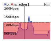
Interface name is shown at the top right, it is trimmed if it's too long (last characters are cut off). The top right corner shows the time interval for the values. Following time values are available:
