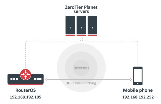
By default, ZeroTier is designed to be zero-configuration. A user can start a new ZeroTier node without having to write configuration files or provide the IP addresses of other nodes. It's also designed to be fast. Any two devices in the world should be able to locate each other and communicate almost instantly so the following example will enable ZeroTier on RouterOS device and connect one mobile phone using the ZeroTier application.
