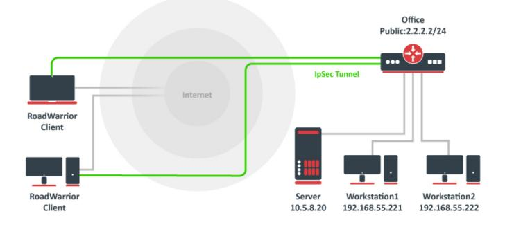
A tunnel is established, a local mode-config IP address is received and a set of dynamic policies are generated.
