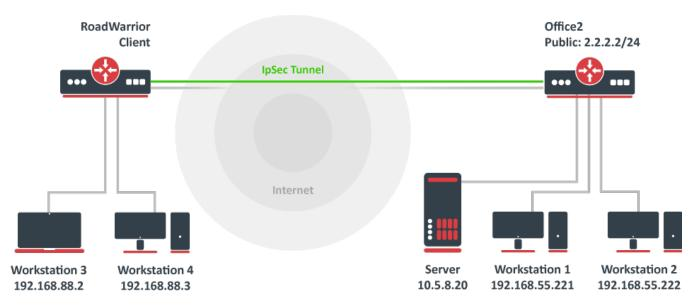
For example, we have a local network 192.168.88.0/24 behind the router and we want all traffic from this network to be sent over the tunnel. First of all, we have to make a new IP/Firewall/Address list which consists of our local network
