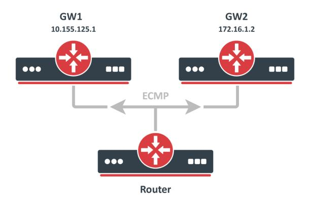
ECMP (Equal cost multi-path) routes have multiple gateways (next-hop) values. All reachable next-hops are copied to FIB and are used to forward packets.
