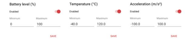
You have an option to log 3 parameters: 1) Battery level; 2) Temperature; 3) Acceleration.
