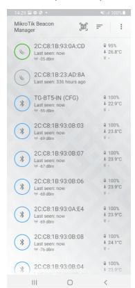
If the list is empty, it means that all the nearby tags are in factory-sleep mode. Once the tag is in advertising or configuration mode, it will show up on the list. To wake up the tag from the factory sleep mode, put the magnet over the tag (activate the reed-switch) for 3-10 seconds.
