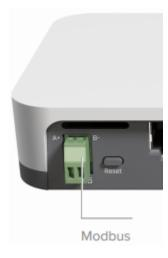
It is important to note that both pins should not be mixed up. Inverting the "A" and "B" connections (incorrect polarisation) will result in communication failure.
