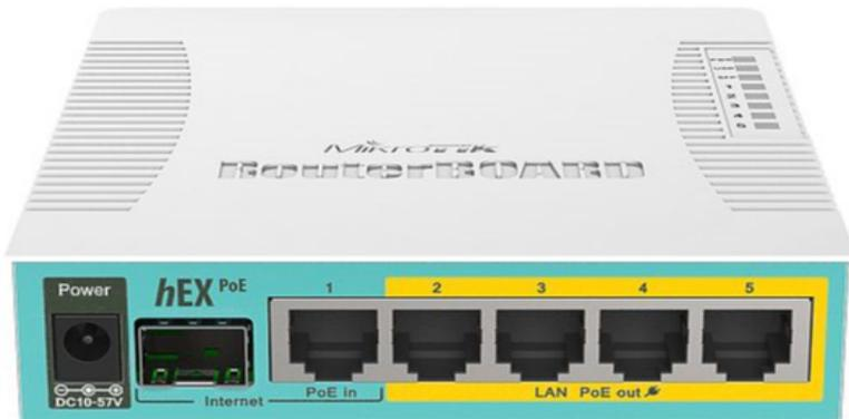
hEX PoE is a powerful five-port Gigabit Ethernet router with an SFP port capable of powering other devices.
