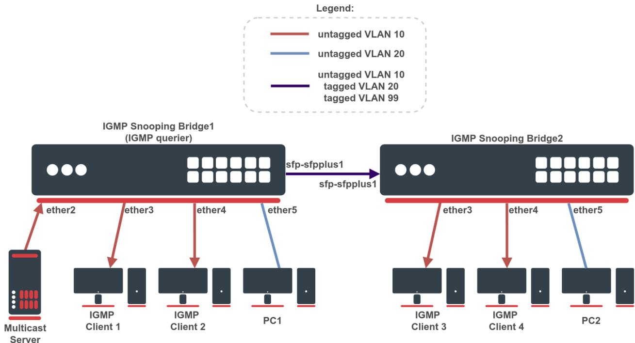
First, create a bridge on both devices and add needed interfaces as bridge ports. To change untagged VLAN for a bridge port, use the `pvid` setting. The Bridge1 will be acting as an IGMP querier. Below are configuration commands for the Bridge1:
