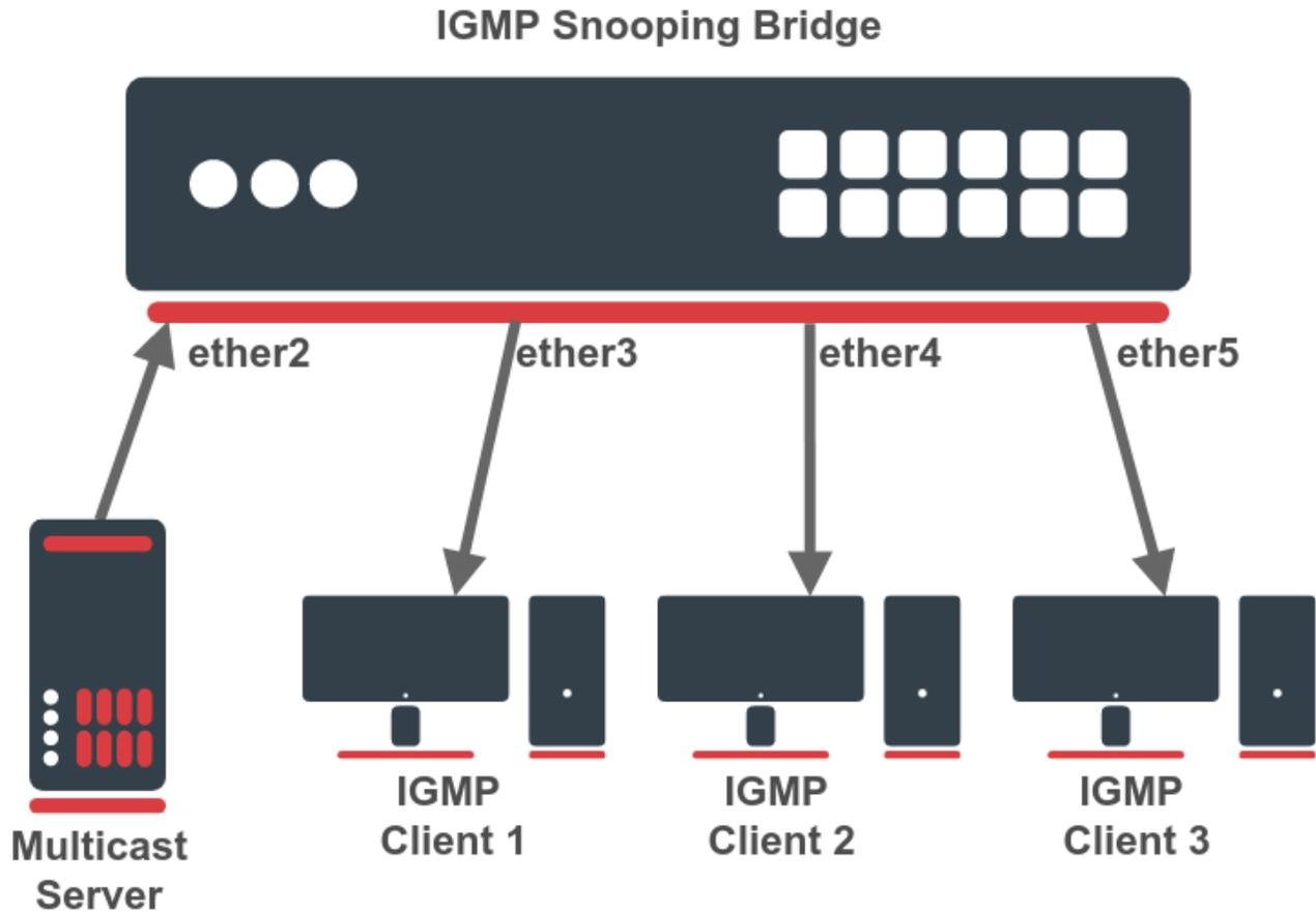
First, create a bridge interface with enabled IGMP snooping. In this example, there is no active IGMP querier (no multicast router or proxy), so a local IGMP querier must be enabled on the same bridge. This can be done with a `multicast-querier` setting. If there is no active IGMP querier in the LAN, the unregistered IP multicast will be flooded and multicast entries will always timeout from the multicast database.
