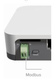
It is important to note that both pins should not be mixed up. Inverting the "A" and "B" connections (incorrect polarisation) will result in communication failure.
