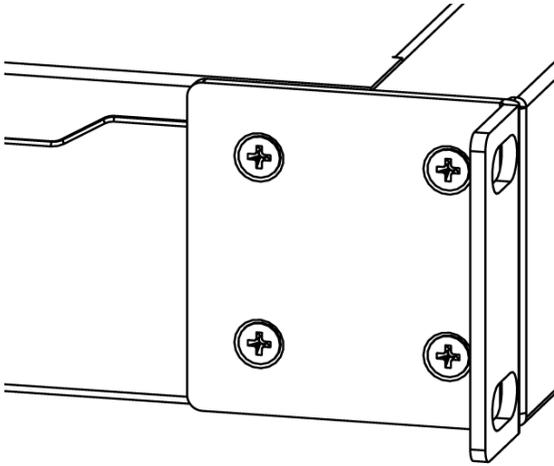
1. Attach rack ears to both sides of the device and tighten four screws to secure them in place, as shown in the picture.
