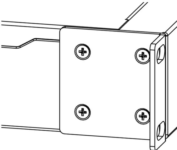
1. Attach rack ears to both sides of the device and tighten four screws to secure them in place, as shown on the picture to the right;
